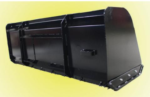
Our decades of expertise designing and manufacturing blades are on display in every part of the design. The ripple-formed moldboard keeps the load moving forward, making for easy work. Large side plates are designed to give this blade a larger capacity, meaning more snow can be moved at a time, and the design also keeps that material visible and easy to monitor. Frame reinforcement gussets between the backplate and side plates mean the blade will stand up to the heaviest snow and ice.
