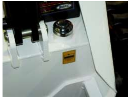
Figure 29: Oil Fill Location
