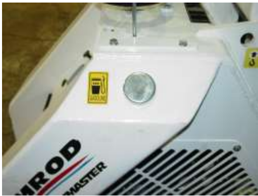
Figure 28: Fuel Fill Location
