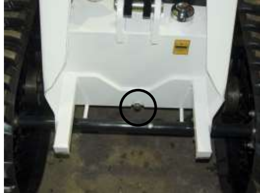
Figure 30: Hydraulic Oil Drain
