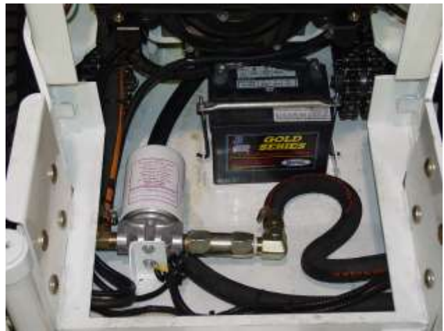
Figure 27: Hydraulic Filter and Battery
